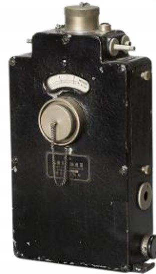
Optical Gas Indicator Model 3 (1939)
